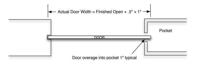
Finished Jamb usually includes slot for door to recess into .5"
