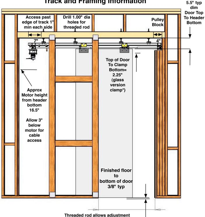
up and down. Average distance from door top to header bottom is 5.5".
