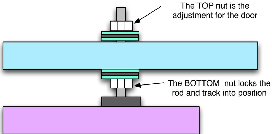
NOTE: Leave the bottom nuts on the threaded rod loose until the top nuts have been adjusted to set the door in both open and closed positions.
