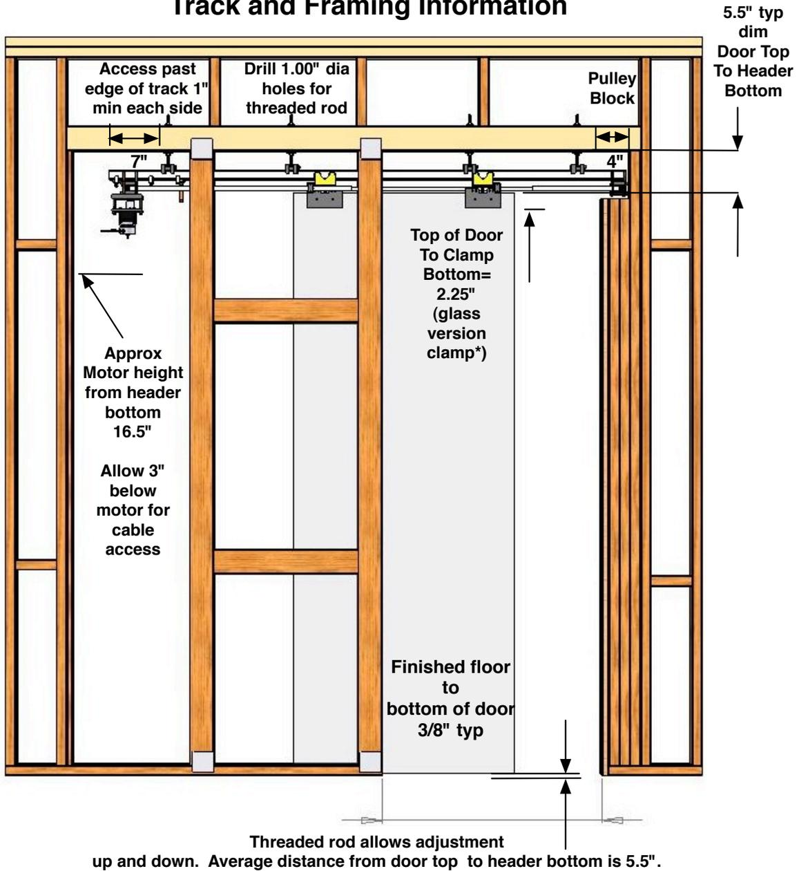
Framing is for illustration purposes only. Glass Clamp Version Shown. \*Wood Clamp mounts on top of door only.
